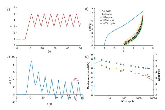
FIG. 4. Elastocaloric effect of polyurethane during triangular solicitation when λ was varied between 3 and 5 at f=0.2Hz. (a) Elongation program. (b) Temperature variation as a function of time. (c) Stress/elongation curves of TPU for a varying number of cycles. (d) Maximum stress and peak-to-peak temperature variation as a function of the number of cycles.
