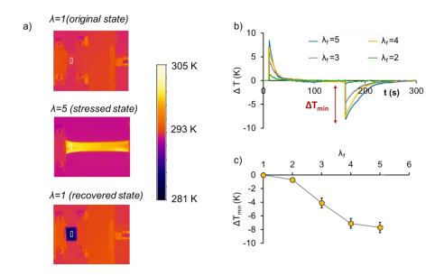
FIG. 3. Elastocaloric properties of polyurethane. (a) IR images for three states:  $\lambda$ =1 (original state),  $\lambda$ =5 (stressed state) and  $\lambda$ =1 (recovered state) of TPU (b) Temperature variation as a function of time ( $\Delta$ T= T(t)-T<sub>room</sub>). (c) The minimum temperature variation  $\Delta$ T<sub>min</sub> as a function of the final elongation  $\lambda_f$ ..
