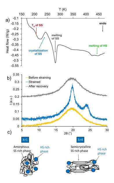
FIG. 1. (a) DSC thermogram of TPU. (b) X-ray diffractograms of TPU before, during and after straining at  $\lambda$ =4. (c) Schematic of strain-induced crystallization of TPU
