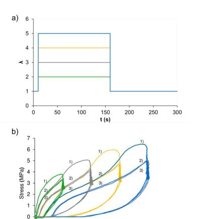
FIG. 2. Mechanical testing of TPU. (a) The mechanical stress program. (b) The evolution of the stress as a function of elongation (first 3 cycles).
